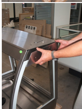
Step 5. Remove One End Trim By Un-doing Screws
