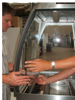
Step 5. Remove One End Trim By Un-doing Screws
