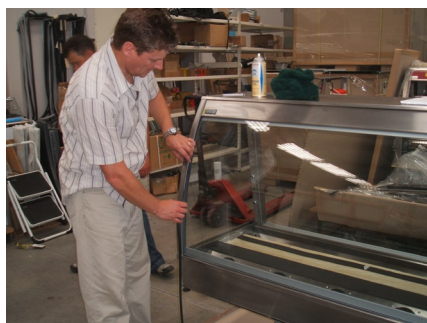
Step 12. Fit Rubber Trim (Supplied) To Front To Secure Glass
