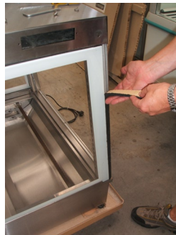
Step 7. Remove Rubber In Fill At Back Of Glass End Panel
