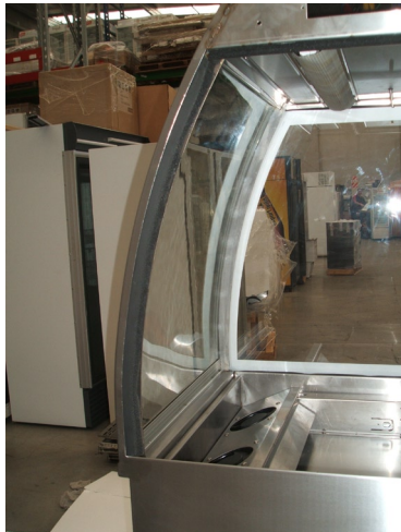
Step 11. Glass in place - Position With Equal Gap At Each End
