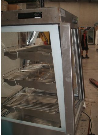
Step 14. Reassemble. 1 - End Glass Panel In-Slide Forward 2 - Rubber Trim Down Edge Of Glass 3 - Install Rear Column Cover 4 - Install End Trim
