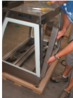
Step 6. Remove One Rear Column Cover By Un-doing Screws
