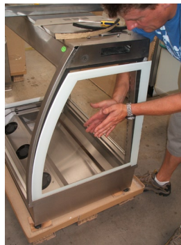
Step 8. Slide End Glass Back To Release And Remove
